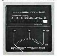
attenuator system is used (OPTI-RANGE). With this feature, you need only set a single range control for an on-scale indication. A second control is provided for situations where the automatic system may not be suitable, as with some measurements of transient signals.
